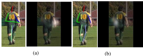
Figure 5. Compared result of global network and the proposed method. (a) Global network, (b) Global(14)-local network. For both (a) and (b), the left image shows the position of body parts and the right image is the original image overlapped with the heatmap of the left wrist.
