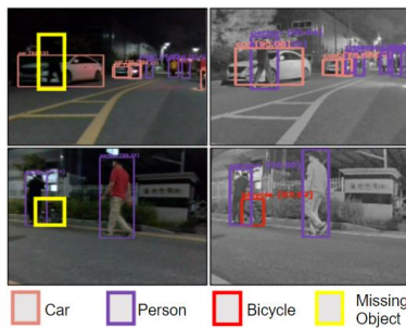
[Fig. 4] Qualitative results. The left column shows the detection results using RGB images, and the right column shows the results using RGB and Nightvision together. Note that using only RGB at night leads to missing objects (yellow rectangles).
