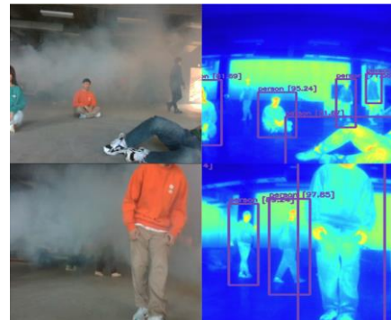
[Fig. 1] Fire situation simulation. The left column shows RGB images, and the right column shows thermal images and the object detection results using the thermal images. Unlike in RGB images, where the field of view is limited due to the smoke, thus humans are not visible, in thermal images, the shape of humans are relatively well revealed.
