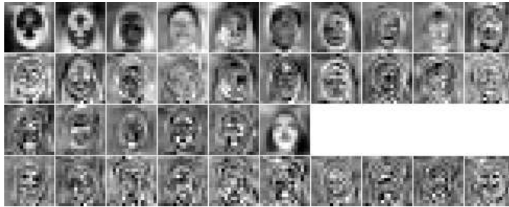
Figure 4.21: Weights of various subspace methods for JAFFE dataset. (1st row: PCA (Eigenfaces), 2nd row: ICA, 3rd row: LDA (Fisherfaces), 4th row: ICA-FX)
