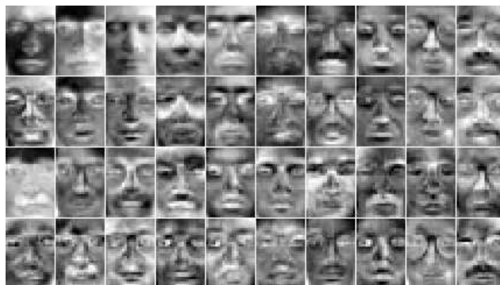
Figure 4.11: Weights of various subspace methods for Yale dataset. (1st row: PCA (Eigenfaces), 2nd row: ICA, 3rd row: LDA (Fisherfaces), 4th row: ICA-FX)
